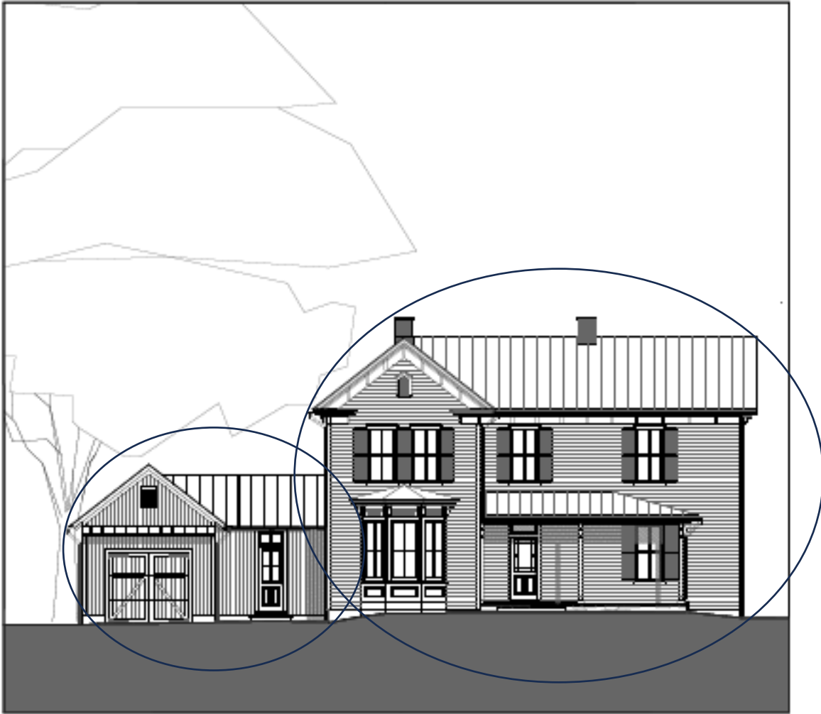
Figure 3. As prescribed in the Design Guidelines, the proposed extension is subordinate to the main house in size and repeats its general patterns with differentiation of detail.
