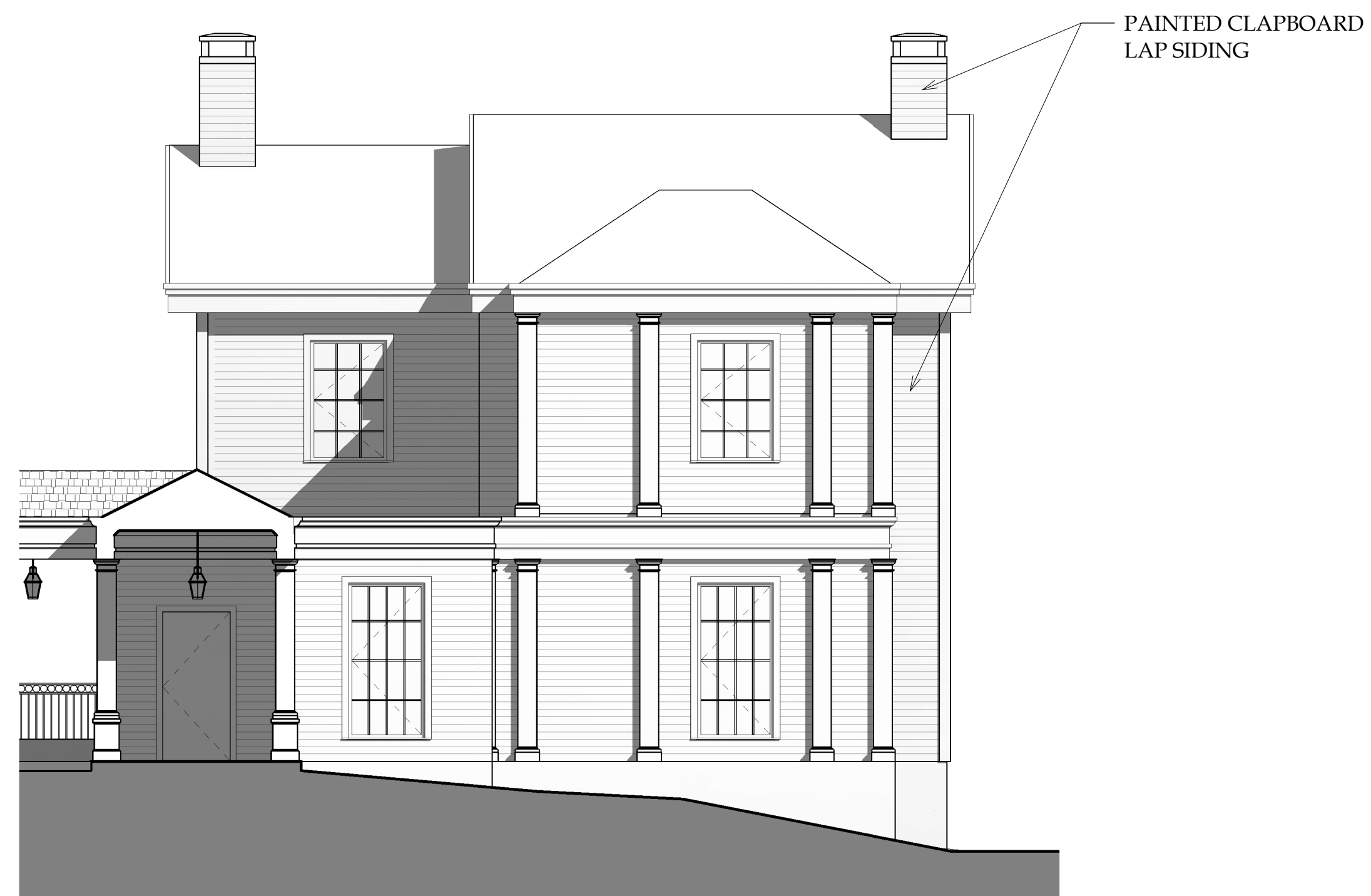
① BLUE HOUSE - WEST ELEVATION 3/16" = 1'-0"
