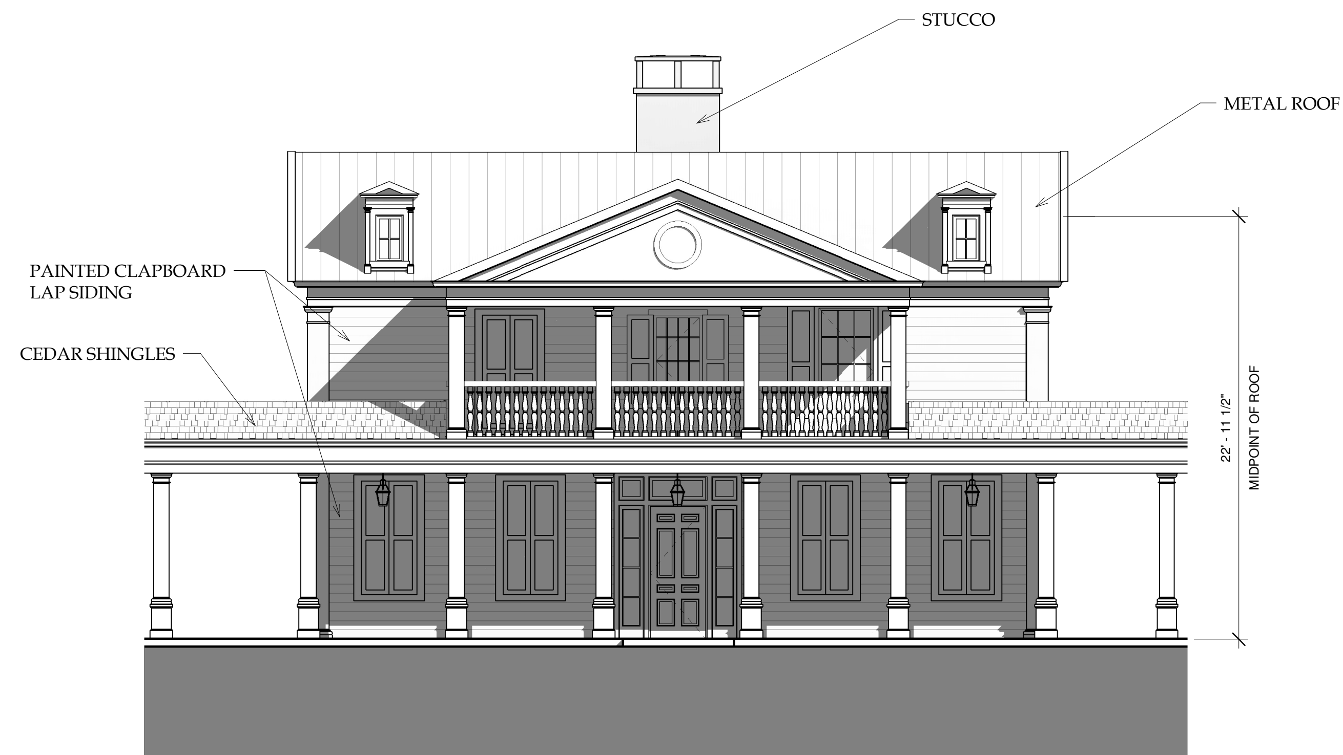
① COURTYARD HOUSE - WEST ELEVATION 3/16" = 1'-0"
