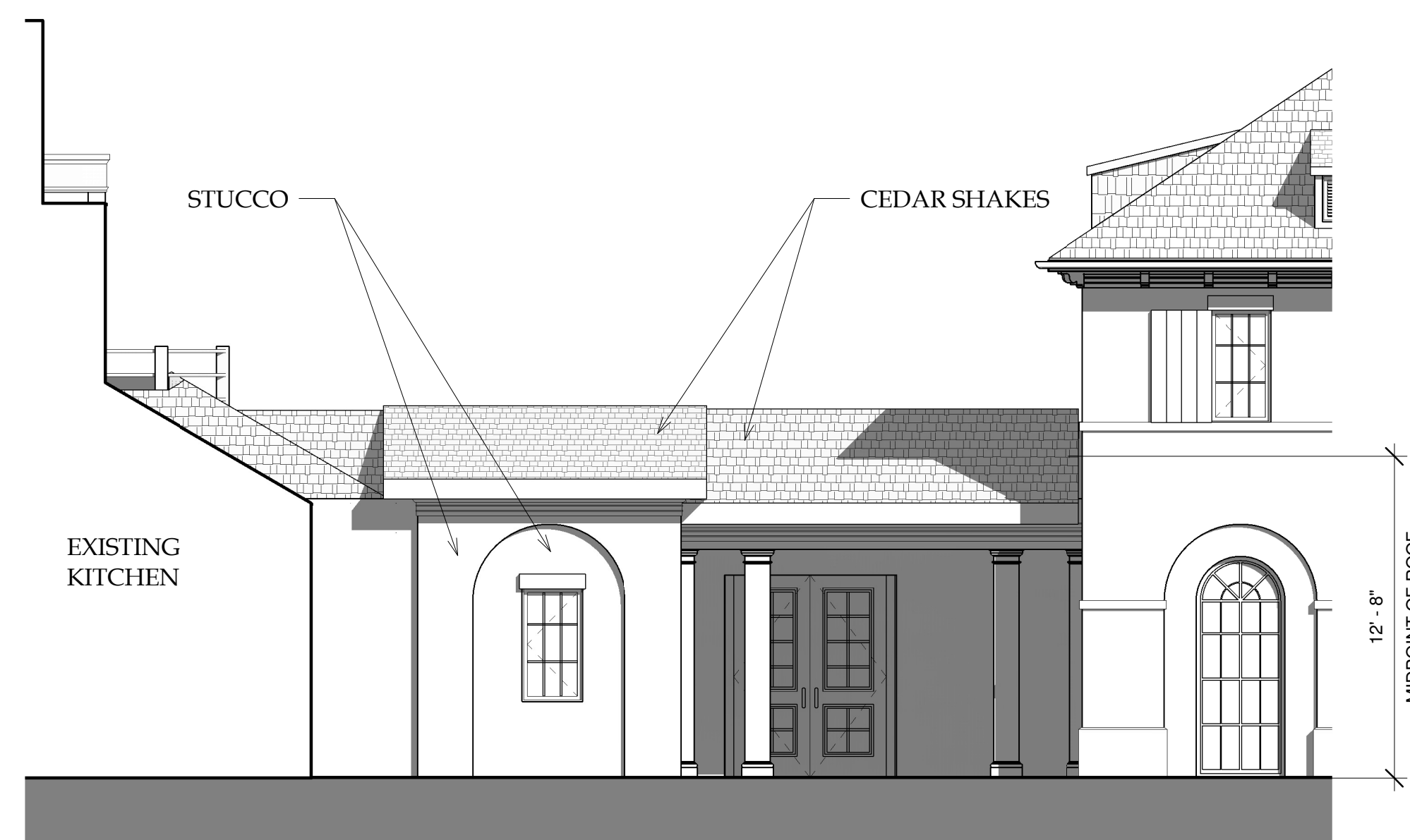
① LINK BUILDING - SOUTH ELEVATION 3/16" = 1'-0"
