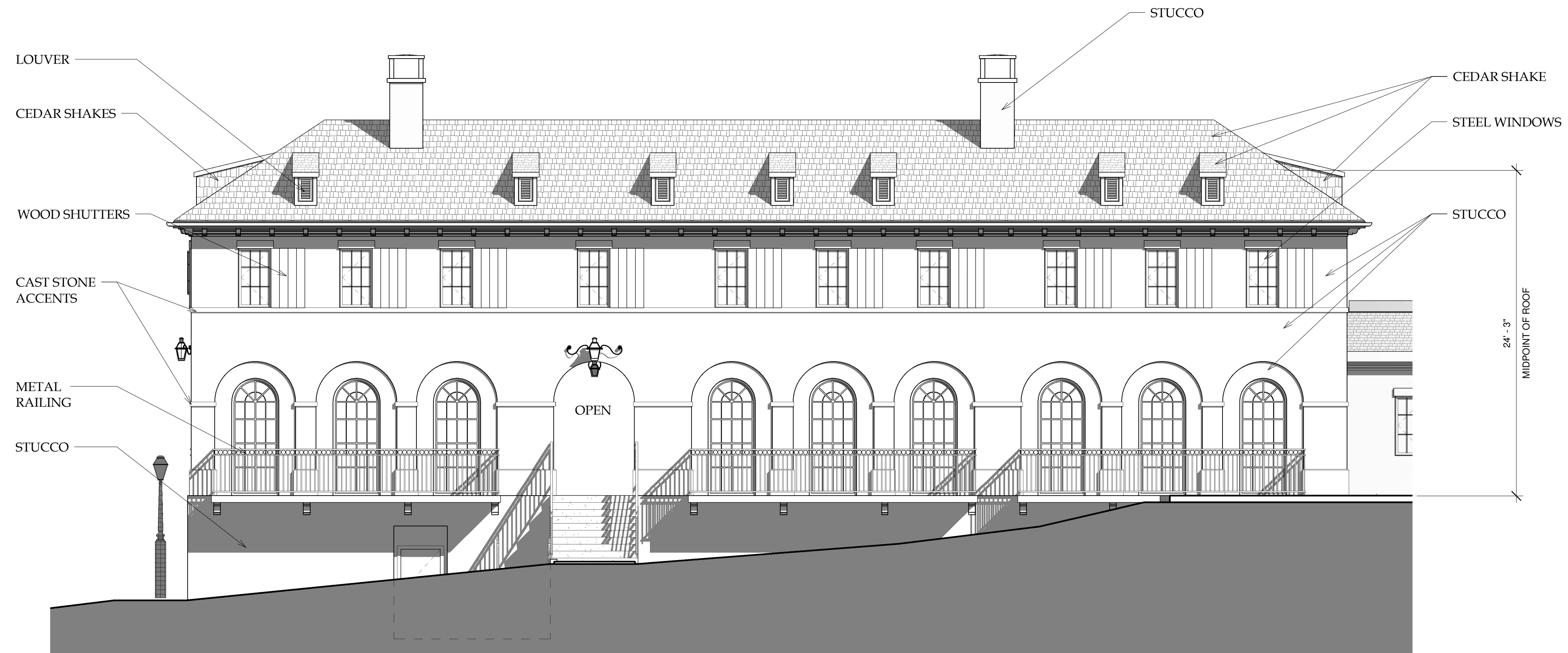
① CARRIAGE HOUSE - NORTH ELEVATION 3/16" = 1'-0"
